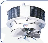
**ECOair** Heating- Ventilation Hot Water Coil of **CC** type with radial fan and diffuser of **DRA** type - this type of device is made of eight separate, big and adjustable louvers. Their shape allows to cover the entire height of the air outlet which gives the ability to freely adjust the distance of the suspension. This type of diffuser allows to direct a stream of air to a specific area. You can also close one, two or three blades and in this way reduce air distribution.
